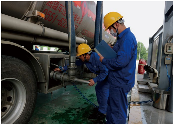
Ⓐ Safety personnel inspecting a tanker vehicle to for leakage hazards of at Feixi Oil Depot
