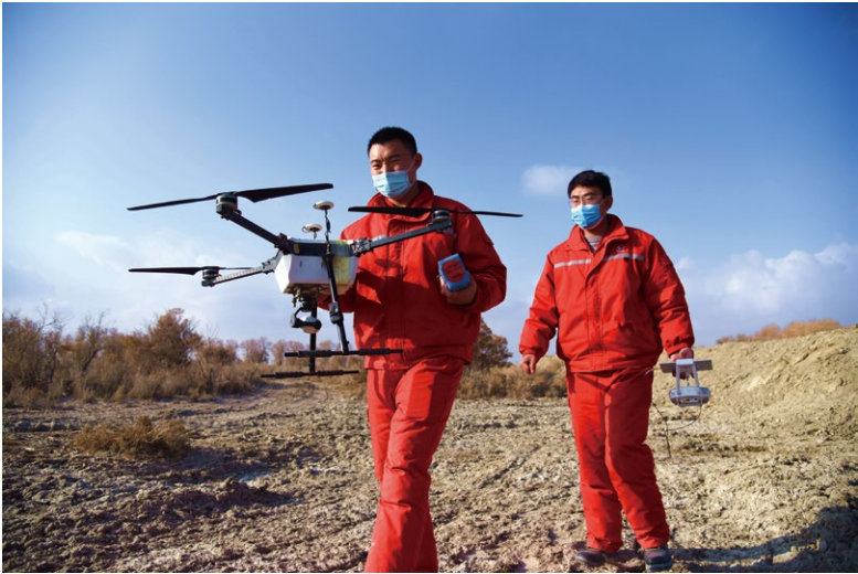
④ The Sky Eye aerial surveillance system uses UAVs for monitoring oil and gas production in winter
